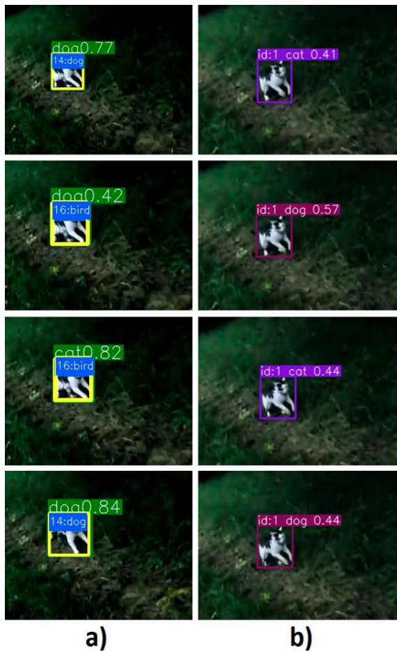
Figure 1. In a) YOLO-NAS and DeepSORT, in b) YOLO11 and BoT-SORT on the Cat video. DeepSORT assigns a new id to the cat when a class change occurs. BoT-SORT can maintain the same id even if an incorrect class detection occurs.
