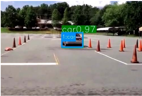
Figure 3. The Car video is the easiest challenge for all detectors and trackers. The car is always detected and tracked perfectly by all algorithms. It is detected as car with very strong confidence scores, and it never loses its tracking identity throughout the entire video.
