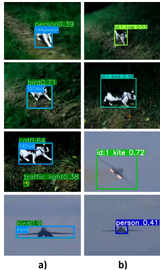
Figure 2. In a) YOLO-NAS and DeepSORT, in b) YOLO11 and BoT-SORT on the Cat video and the Airplane video. The bounding box calculations are remarkably successful and accurate, the tracking is also quite good, however there are too many incorrect class detections both in YOLO-NAS and YOLO11.
